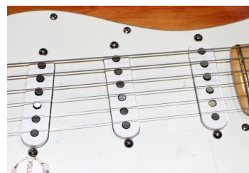
Figure 10.3 Pickups on an electric guitar.
