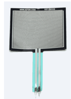
Figure 2.28 A force sensing resistor (FSR).
